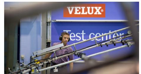
Installation and module watertightness is tested in a wind tunnel with wind speeds up to 37 m/s (hurricane force). The test uses a full installation with modules and flashing.
