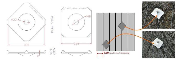
Steelgrid HR high strength geocomposite mesh has been designed to work in combination with a specifically de- veloped anchor plate: the '**Steelgrid HR System Plate**'.
