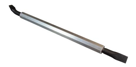
Hollow-shaped crowbar with hexagonal shaft. Used mostly by demounting, mountain demolition, mountain examination of mountain ranges after shot blasting. Both ends have a conical fit for attachment in the shaft.
